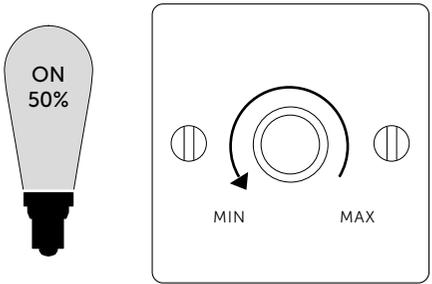
Rotate the knob to program the minimum brightness levels.
