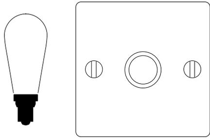
When the lamp is switched **ON**, press and hold **"PUSH KNOB"** for 3-5 sec until the lamps appear at half their brightness level.
