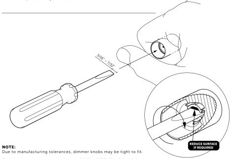
To allow for easier assembly, insert a 3/16" - 7/32" (5 - 5.5mm) flat head screwdriver and rotate 360° to remove excess material from the flat section of the insert.
